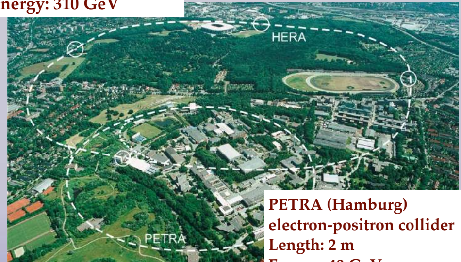
HERA (Hamburg) electron-proton collider Length: 6 km Energy: 310 GeV
