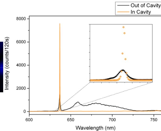
Effect of cavity coupling on NV emission
