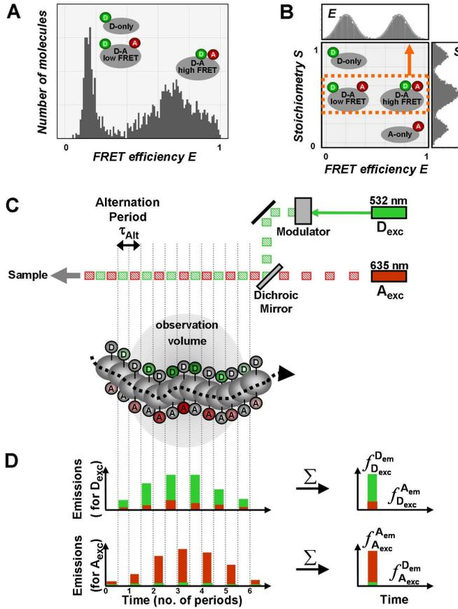
**Figure 1. Alternating-laser excitation spectroscopy of single molecules.**
