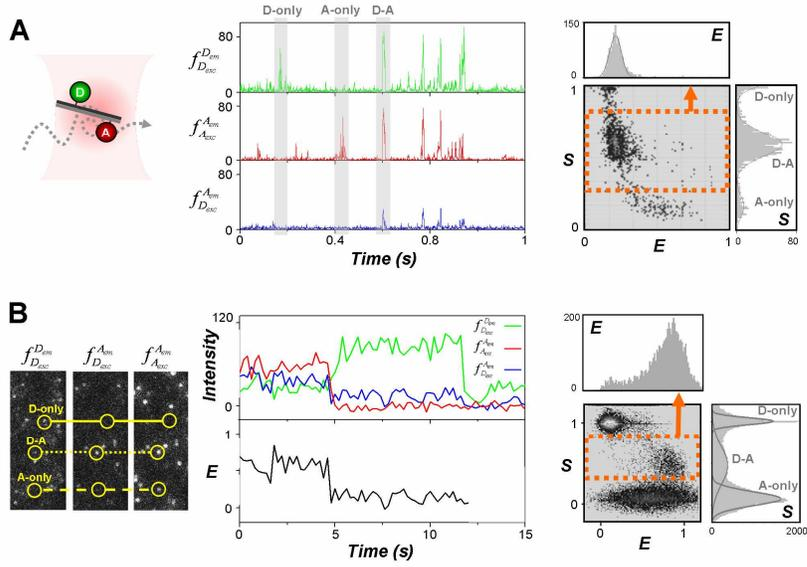
**Figure 2. Implementation of ALEX on diffusing and immobilized molecules**
