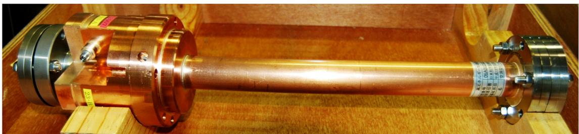
Figure 5.4: Photo of one of the C-band cavity BPMs before installation.
