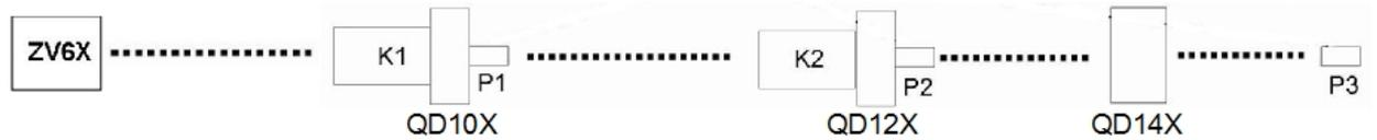
Figure 3.24: Diagram of layout of FONT5 at ATF2. ZV6X is a corrector magnet and QD10X, QD12X and QD14X are quadrupole magnets. P1, P2 and P3 are BPMs and K1 and K2 are kickers (one each for correction in  $y$  and  $y'$ ).
