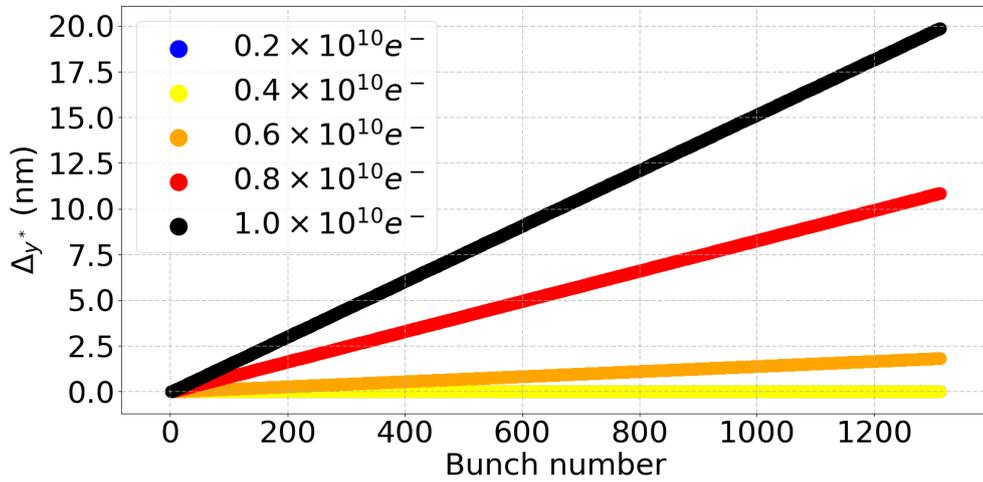
Figure 5.9: Vertical orbit deflection at the IP between the first and last bunch of a train  $\Delta y^*$  vs. bunch number for a train with a constant incoming angle offset of  $0.1\sigma_{y'}$  of the train of bunches in the 250 GeV ILC BDS for 5 beam intensities, calculated with PLACET with resistive wall effects included.
