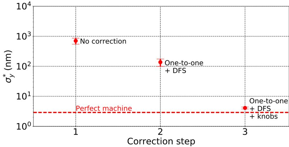
Figure 6.6: Average vertical beam size at the 380 GeV CLIC IP ( $\sigma_y^*$ ) vs. correction step: One-to-one, DFS, WFS corrections and IP tuning knobs. The red dashed line show the vertical beam size at the IP for a perfect machine, 2.9 nm, calculated with PLACET with wakefields.
