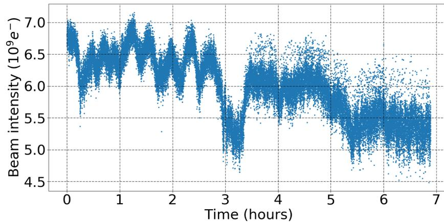
Figure 4.5: ATF2 beam intensity drift, measured by the Integrated Current Transformer located near the IP.
