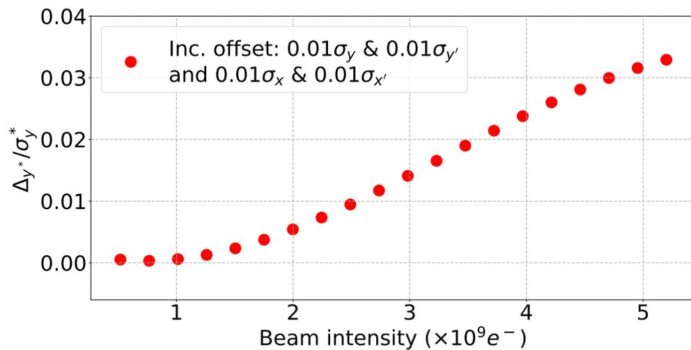
Figure 6.14: Vertical orbit deflection at the IP between the first and last bunch of a train normalised by the IP vertical beam size ( $\Delta y^*/\sigma_y^*$ ) vs. beam intensity for a train with incoming constant horizontal position and angle offsets of respectively  $0.01\sigma_x$  and  $0.01\sigma_{x'}$  and vertical incoming position and angle offsets of respectively  $0.01\sigma_y$  and  $0.01\sigma_{y'}$  in the 380 GeV CLIC BDS, calculated with PLACET with resistive walls.
