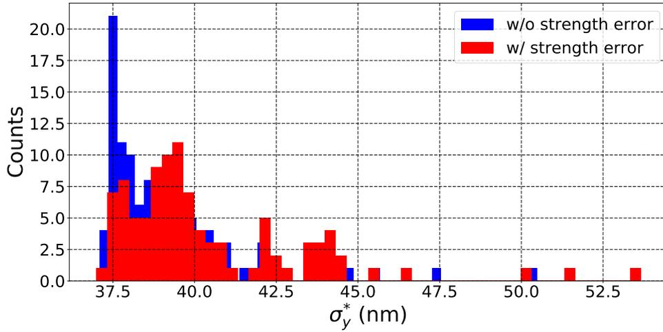
Figure 3.17: Effect of quadrupoles and sextupoles strength error of  $10^{-4}$  RMS at  $1.0 \times 10^{10} e^-$  on the vertical IP beam size ( $\sigma_y^*$ ), in presence of wakefields calculated with PLACET.
