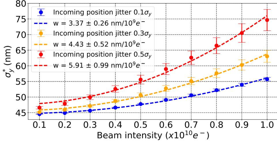
Figure 3.21: Effect of incoming 0.1, 0.3 and 0.5  $\sigma_y$  beam position jitter on the vertical beam size at the IP ( $\sigma_y^*$ ) vs. the beam intensity, calculated with PLACET in the presence of wakefields.
