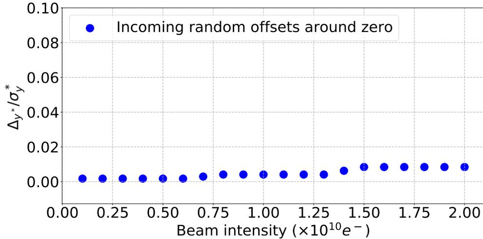
Figure 5.14: Vertical orbit deflection at the IP between the first and last bunch of a train normalised by the IP vertical beam size ( $\Delta y^*/\sigma_y^*$ ) vs. beam intensity for a train with a random and around zero incoming vertical and horizontal position and angle offsets of between  $-0.05$  and  $0.05 \sigma$  in the 250 GeV ILC BDS, calculated with PLACET with resistive wall effects included.
