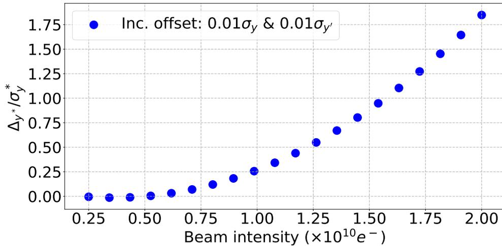
Figure 5.11: Vertical orbit deflection at the IP between the first and last bunch of a train normalised by the IP vertical beam size ( $\Delta y^*/\sigma_y^*$ ) vs. beam intensity for a train with incoming constant position and angle offsets of respectively  $0.01\sigma_y$  and  $0.01\sigma_{y'}$  in the 250 GeV ILC BDS, calculated with PLACET with resistive wall effects included.
