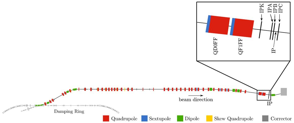
Figure 2.11: Schematic of the ATF2 beamline showing the positions of the IP-BPMs.
