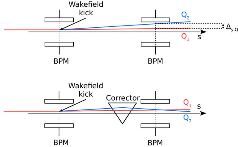
Figure 3.14: Schematic of the Wakefields Free Steering corrections.
