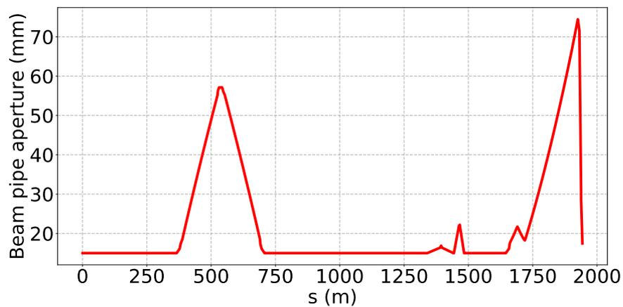
Figure 6.8: The CLIC BDS beam aperture profile.
