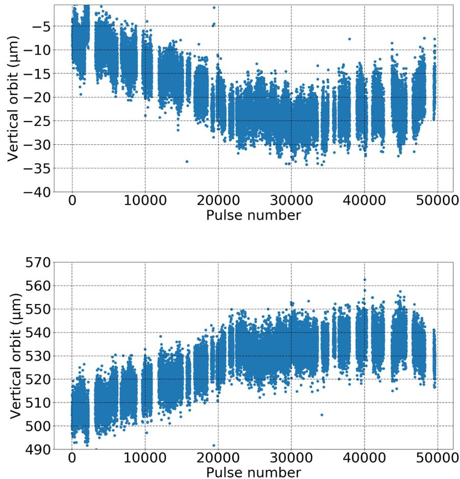
Figure 4.4: Vertical orbit at 2 selected BPMs: QD10AFF and QF9AFF. 50000 pulses travel in ATF2 in 4h27.
