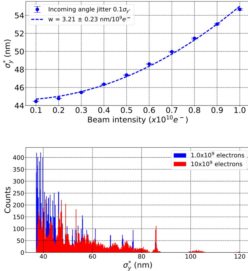
Figure 3.19: (Top) Effect of an incoming  $0.1\sigma_{y'}$  beam angle jitter on the vertical beam size at the IP ( $\sigma_y^*$ ) vs. the beam intensity; (Bottom) distributions of the vertical beam size at the IP ( $\sigma_y^*$ ) for low and high beam intensities, calculated with PLACET in the presence of wakefields.
