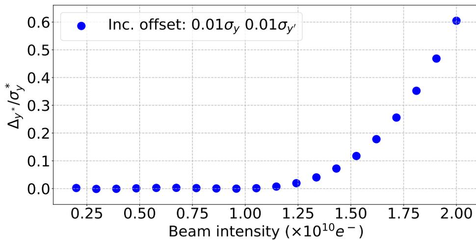
Figure 5.23: Vertical orbit deflection at the IP between the first and last bunch of a train normalised by the IP vertical beam size ( $\Delta y^*/\sigma_y^*$ ) vs. beam intensity for a train with incoming constant position and angle offsets of respectively  $0.01\sigma_y$  and  $0.01\sigma_{y'}$  in the 500 GeV ILC BDS, calculated with PLACET with resistive wall effects included.
