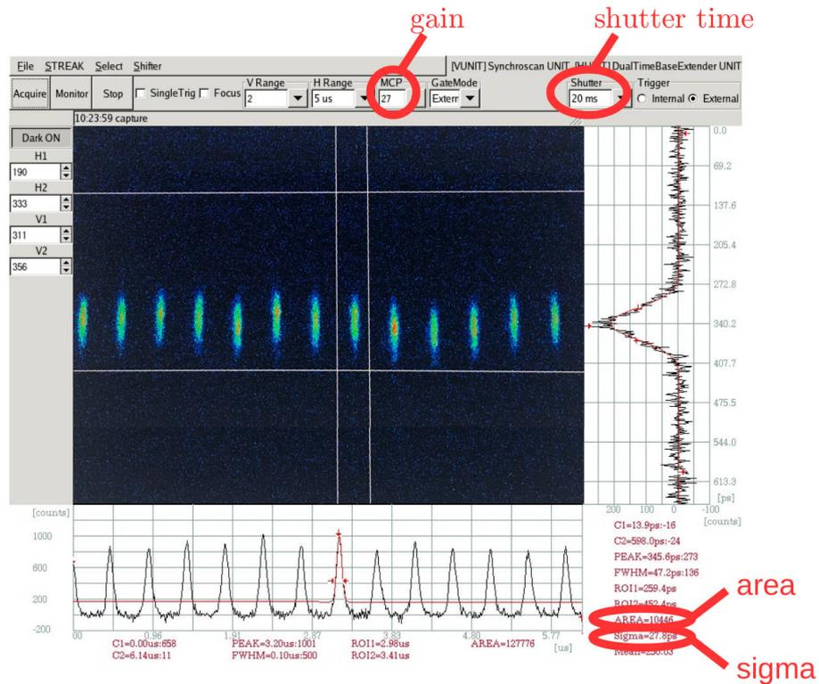
Figure 4.2: Screenshot of the software used for the ATF2 bunch length measurement. The gain, shutter time and area parameters are shown for the measurement. The longitudinal profile of consecutive bunches is shown at the bottom of the figure. The bunch length, sigma is in ps.
