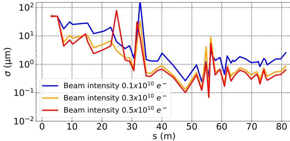
Figure 4.11: BPM vertical resolutions along the beamline.
