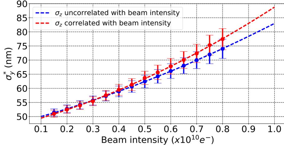
Figure 3.31: Simulations of the impact of the ATF2 bunch length ( $\sigma_z$ ) on the vertical IP beam size ( $\sigma_y^*$ ) vs. the beam intensity, calculated with PLACET in the presence of wakefields.
