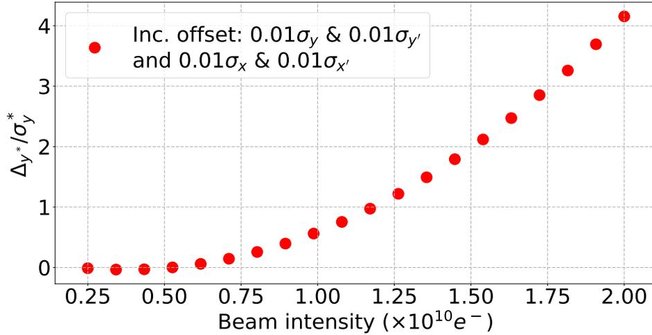
Figure 5.12: Vertical orbit deflection at the IP between the first and last bunch of a train normalised by the IP vertical beam size ( $\Delta y^*/\sigma_y^*$ ) vs. beam intensity for a train with incoming constant horizontal position and angle offsets of respectively  $0.01\sigma_x$  and  $0.01\sigma_{x'}$  and vertical incoming position and angle offsets of respectively  $0.01\sigma_y$  and  $0.01\sigma_{y'}$  in the 250 GeV ILC BDS, calculated with PLACET with resistive wall effects included.
