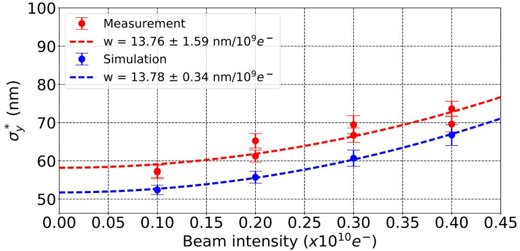
Figure 4.26: Comparison between measurements and simulations of the vertical beam size at the IP ( $\sigma_y^*$ ) vs. the beam intensity and the intensity-dependent parameter  $w$ .
