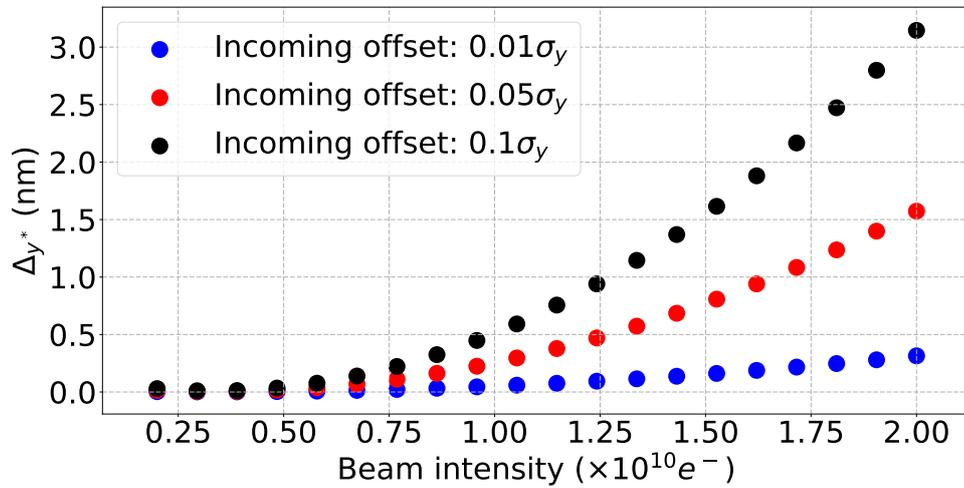
Figure 5.22: Vertical orbit deflection at the IP between the first and last bunch of a train  $\Delta y^*$  vs. beam intensity for three incoming constant position offsets of the train of bunches in the 500 GeV ILC BDS:  $0.01\sigma_y$ ,  $0.05\sigma_y$  and  $0.1\sigma_y$ , calculated with PLACET with resistive wall effects included.
