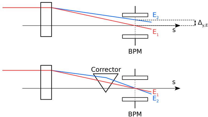
Figure 3.13: Schematic of the Dispersion Free Steering correction.
