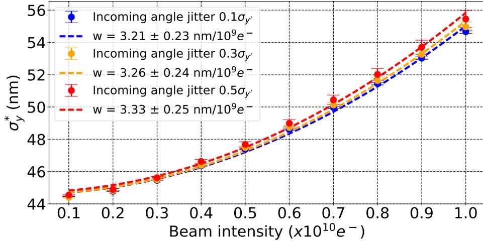
Figure 3.22: Effect of incoming 0.1, 0.3 and 0.5  $\sigma_{y'}$  beam angle jitter on the vertical beam size at the IP ( $\sigma_y^*$ ) vs. the beam intensity, calculated with PLACET in the presence of wakefields.
