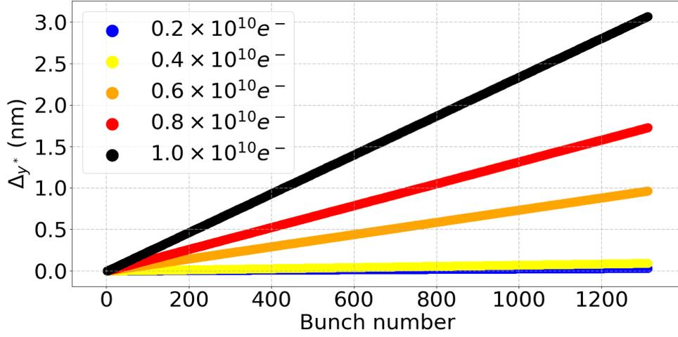
Figure 5.8: Vertical orbit deflection at the IP between the first and last bunch of a train  $\Delta y^*$  vs. bunch number for a train with a constant incoming position offset of  $0.1\sigma_y$  of the train of bunches in the 250 GeV ILC BDS for 5 beam intensities, calculated with PLACET with resistive wall effects included.
