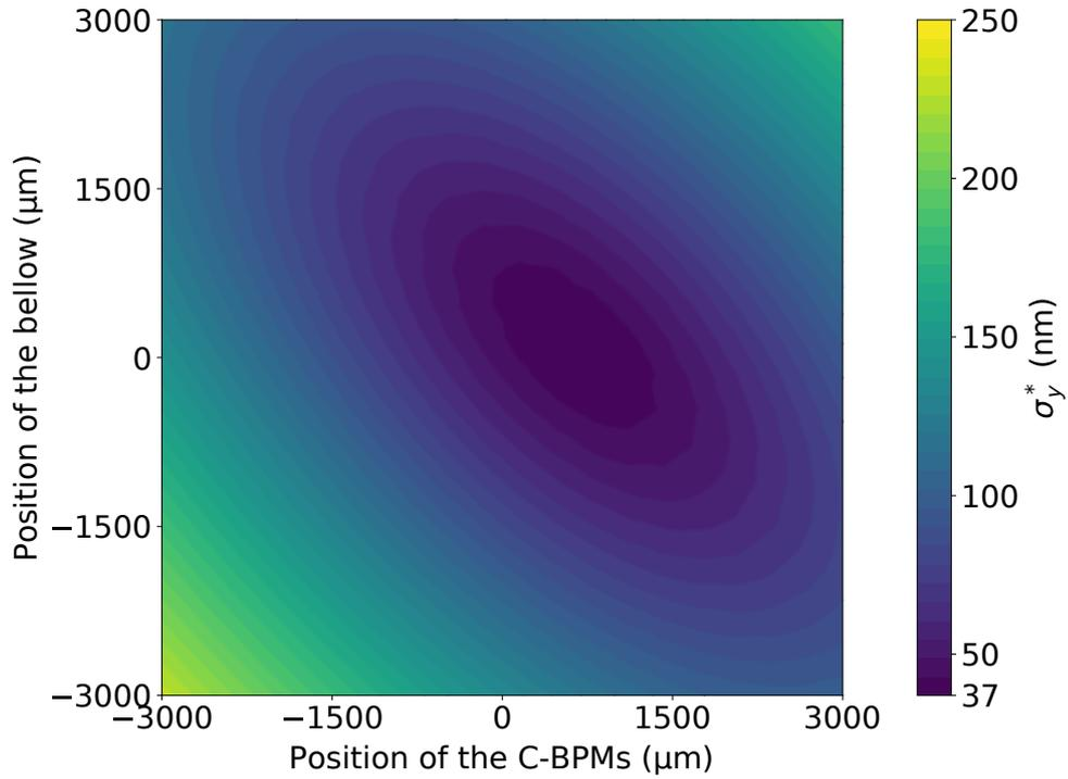
Figure 3.28: Contour plot of the simulation of the impact of the position of the C-BPMs and the bellows on the vertical beam size at the IP  $\sigma_y^*$ , for one machine, calculated with PLACET in the presence of wakefields.
