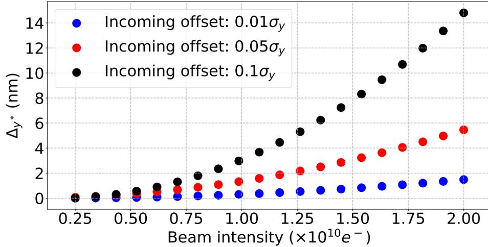
Figure 5.10: Vertical orbit deflection at the IP between the first and last bunch of a train  $\Delta y^*$  vs. beam intensity for three incoming constant position offsets of the train of bunches in the 250 GeV ILC BDS:  $0.01\sigma_y$ ,  $0.05\sigma_y$  and  $0.1\sigma_y$ , calculated with PLACET with resistive wall effects included.
