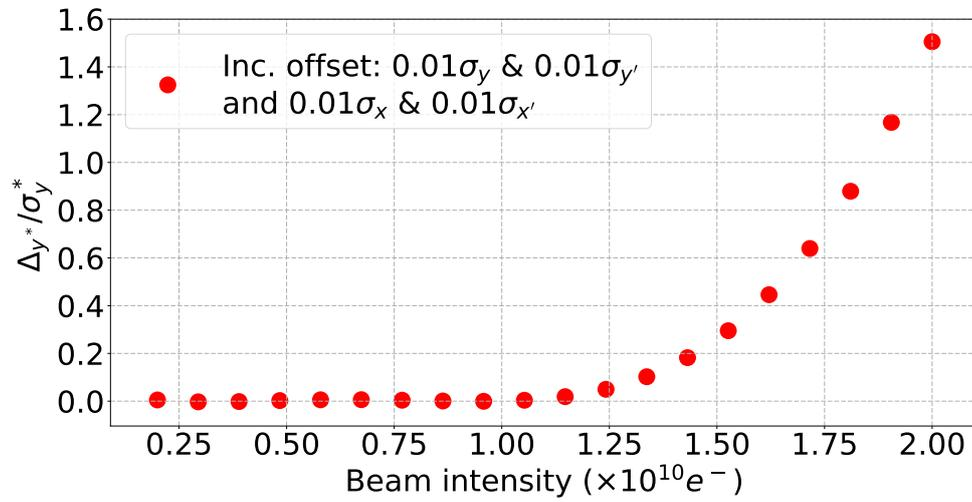
Figure 5.24: Vertical orbit deflection at the IP between the first and last bunch of a train normalised by the IP vertical beam size ( $\Delta y^*/\sigma_y^*$ ) vs. beam intensity for a train with incoming constant horizontal position and angle offsets of respectively  $0.01\sigma_x$  and  $0.01\sigma_{x'}$  and vertical incoming position and angle offsets of respectively  $0.01\sigma_y$  and  $0.01\sigma_{y'}$  in the 500 GeV ILC BDS, calculated with PLACET with resistive wall effects included.
