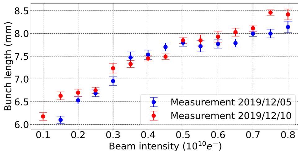
Figure 4.3: Bunch length measurement vs. beam intensity measured on two separate days.
