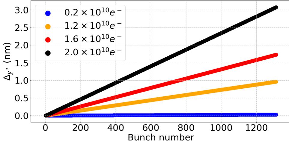
Figure 5.20: Vertical orbit deflection at the IP between the first and last bunch of a train  $\Delta y^*$  vs. bunch number for a train with a constant incoming position offset of  $0.1\sigma_y$  of the train of bunches in the 500 GeV ILC BDS for 5 beam intensities, calculated with PLACET with resistive wall effects included.
