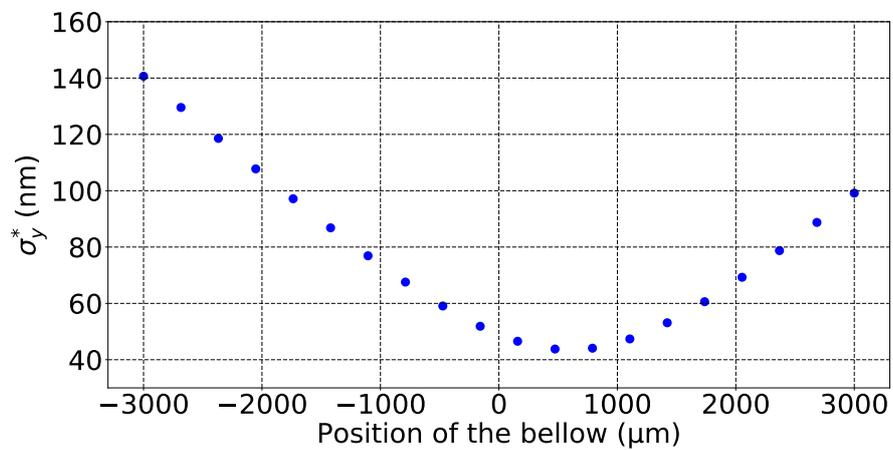
Figure 3.26: Vertical beam size at the IP  $\sigma_y^*$  vs. the position of the bellows, for one machine, calculated with PLACET in the presence of wakefields.
