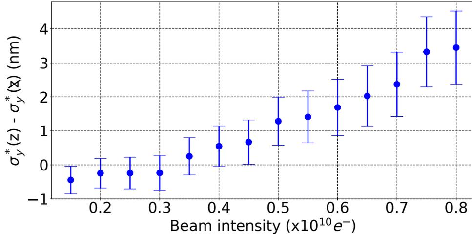
Figure 3.32: Difference between the vertical IP beam size ( $\sigma_y^*$ ) considering the bunch length ( $\sigma_z$ ) is correlated and the vertical IP beam size ( $\sigma_y^*$ ) considering the bunch length ( $\sigma_z$ ) is not correlated with the beam intensity, calculated with PLACET in the presence of wakefields.
