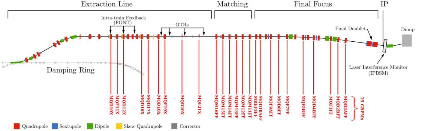
Figure 3.3: Positions of Cavity BPMS in ATF2.
