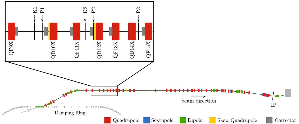
Figure 2.10: Schematic of the ATF2 beamline showing the positions of the upstream FONT BPMs.
