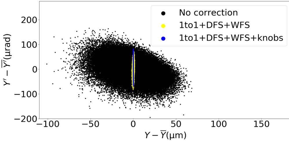
Figure 5.17: Centered vertical phase space at the 500 GeV ILC BDS IP,  $Y' - \bar{Y}'$  vs.  $Y - \bar{Y}$ , for 3 cases: no correction, One-to-one steering, DFS, WFS and One-to-one steering, DFS, WFS and knobs, calculated with PLACET with wakefields.
