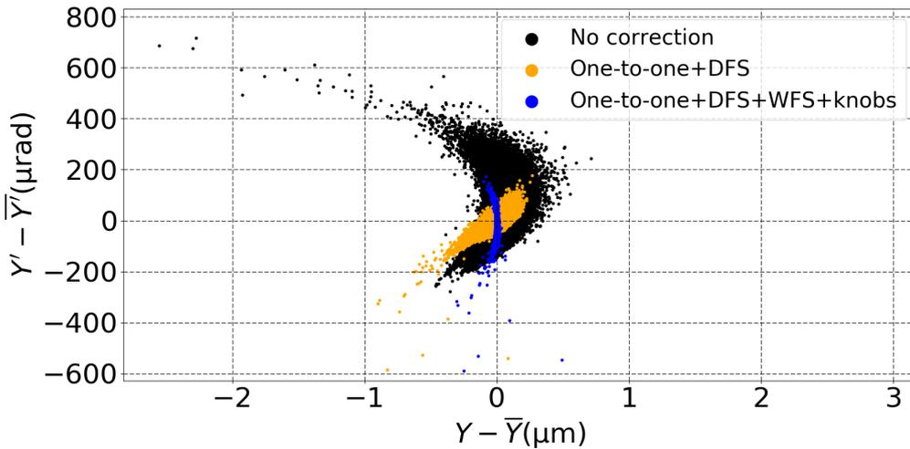
Figure 6.5: Centered vertical phase space at the 380 GeV CLIC BDS IP,  $Y' - \bar{Y}'$  vs.  $Y - \bar{Y}$ , for 3 cases: no correction, One-to-one steering, DFS, WFS and One-to-one steering, DFS, WFS and knobs, calculated with PLACET with wakefields.
