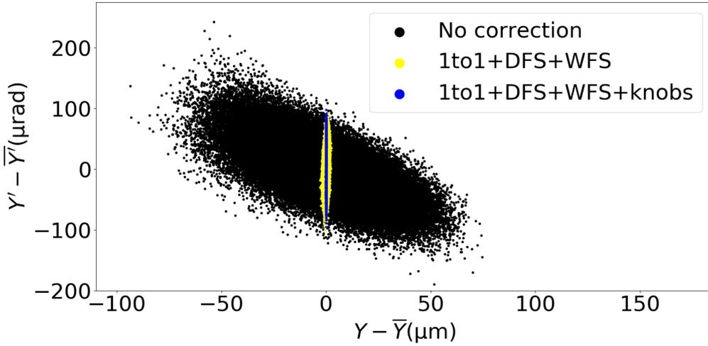
Figure 5.3: Centered vertical phase space at the 250 GeV ILC BDS IP,  $Y' - \bar{Y}'$  vs.  $Y - \bar{Y}$ , for 3 cases: no correction, One-to-one steering, DFS, WFS and One-to-one steering, DFS, WFS and knobs, calculated with PLACET with wakefields.
