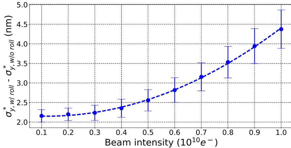
Figure 3.18: Effect of 200  $\mu$ rad RMS rolls of BPMs, quadrupoles and sextupoles on the vertical IP beam size ( $\sigma_y^*$ ) vs. the beam intensity, in presence of wakefields calculated with PLACET.
