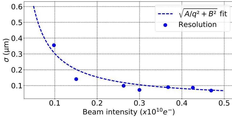
Figure 4.10: Vertical resolution vs. beam intensity for BPM MQD4AFF, a cavity BPM.
