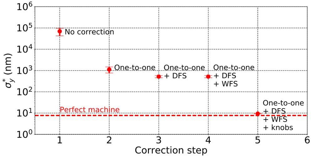
Figure 5.4: Average vertical beam size at the 250 GeV ILC IP ( $\sigma_y^*$ ) vs. correction step: One-to-one, DFS, WFS corrections and IP tuning knobs. The red dashed line show the vertical beam size at the IP for a perfect machine, 7.7 nm.
