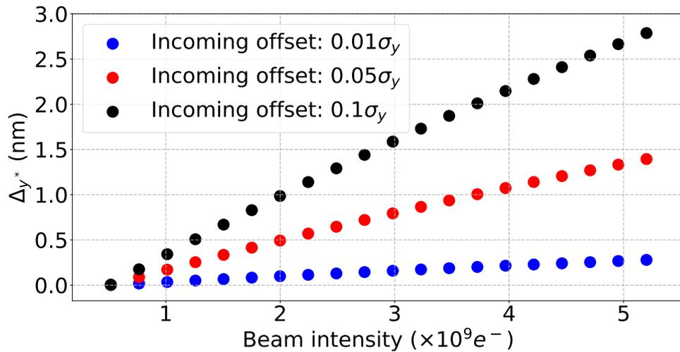
Figure 6.12: Vertical orbit deflection at the IP between the first and last bunch of a train  $\Delta y^*$  vs. beam intensity for three incoming constant position offsets of the train of bunches in the 380 GeV CLIC BDS:  $0.01\sigma_y$ ,  $0.05\sigma_y$  and  $0.1\sigma_y$ , calculated with PLACET with resistive walls.
