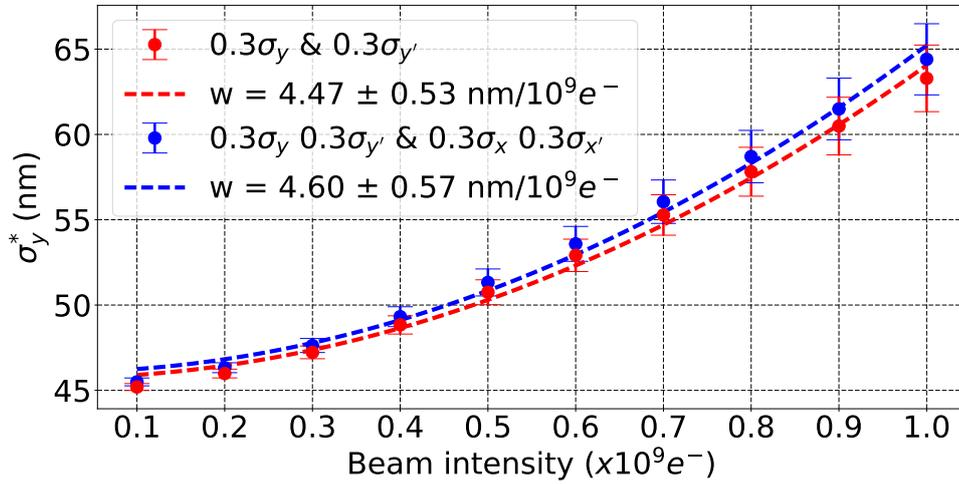
Figure 3.24: Effect of incoming horizontal position and angle jitters of respectively  $0.3\sigma_x$  and  $0.3\sigma_{x'}$  and incoming vertical position and angle jitters of respectively  $0.3\sigma_y$  and  $0.3\sigma_{y'}$  on the vertical beam size at the IP ( $\sigma_y^*$ ) vs. the beam intensity, calculated with PLACET in the presence of wakefields.
