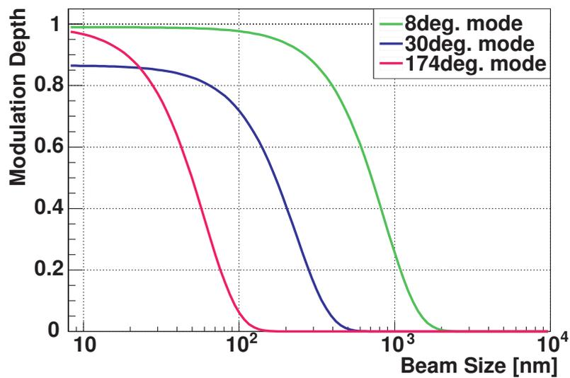
Figure 2.7: Dynamic ranges of the ATF2 IPBSM [4]
