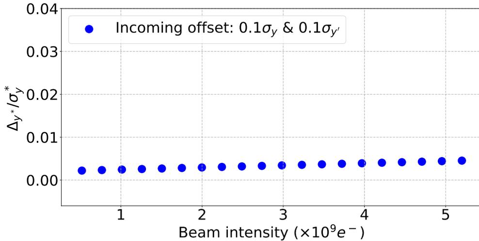
Figure 6.15: Vertical orbit deflection at the IP between the first and last bunch of a train normalised by the IP vertical beam size ( $\Delta y^*/\sigma_y^*$ ) vs. beam intensity for a train with a random and around zero incoming vertical and horizontal position and angle offsets of between -0.05 and 0.05  $\sigma$  in the 380 GeV CLIC BDS, calculated with PLACET with resistive walls.
