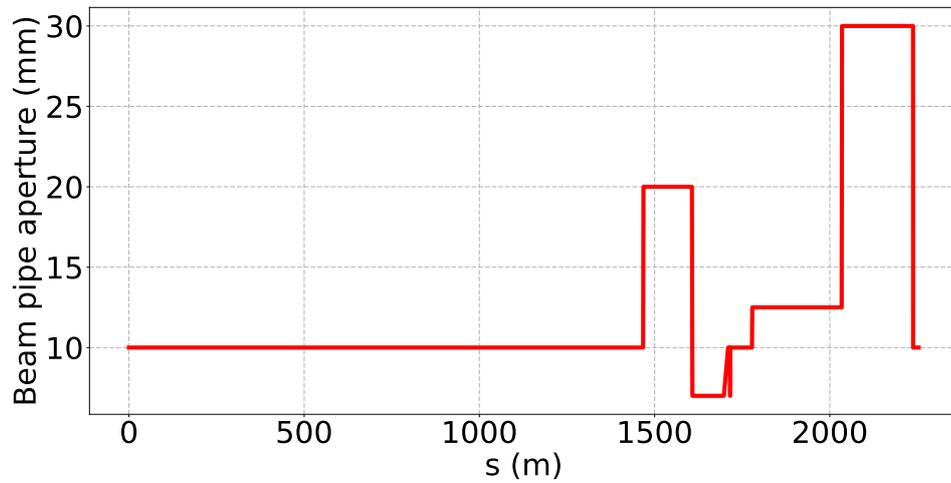
Figure 5.6: The ILC BDS beam aperture profile vs.  $s$ .
