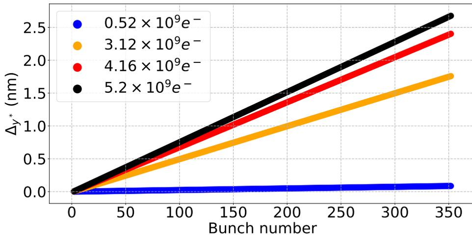
Figure 6.10: Vertical orbit deflection at the IP between the first and last bunch of a train  $\Delta_{y^*}$  vs. bunch number for a train with a constant incoming position offset of  $0.1\sigma_y$  of the train of bunches in the 380 GeV CLIC BDS, calculated with PLACET with resistive walls.
