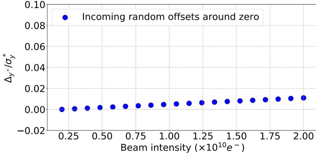
Figure 5.25: Vertical orbit deflection at the IP between the first and last bunch of a train normalised by the IP vertical beam size ( $\Delta y^*/\sigma_y^*$ ) vs. beam intensity for a train with a random and around zero incoming vertical and horizontal position and angle offsets of between  $-0.05$  and  $0.05 \sigma$  in the 500 GeV ILC BDS, calculated with PLACET with resistive wall effects included.
