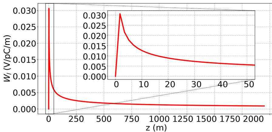
Figure 6.9: The CLIC resistive walls wakepotential for a copper beam pipe with a constant radius of 15 mm for the length of the CLIC BDS ( $\sim 1949$  m). The zoom shows the wakepotential for the length of a train ( $\sim 52.8$  m).
