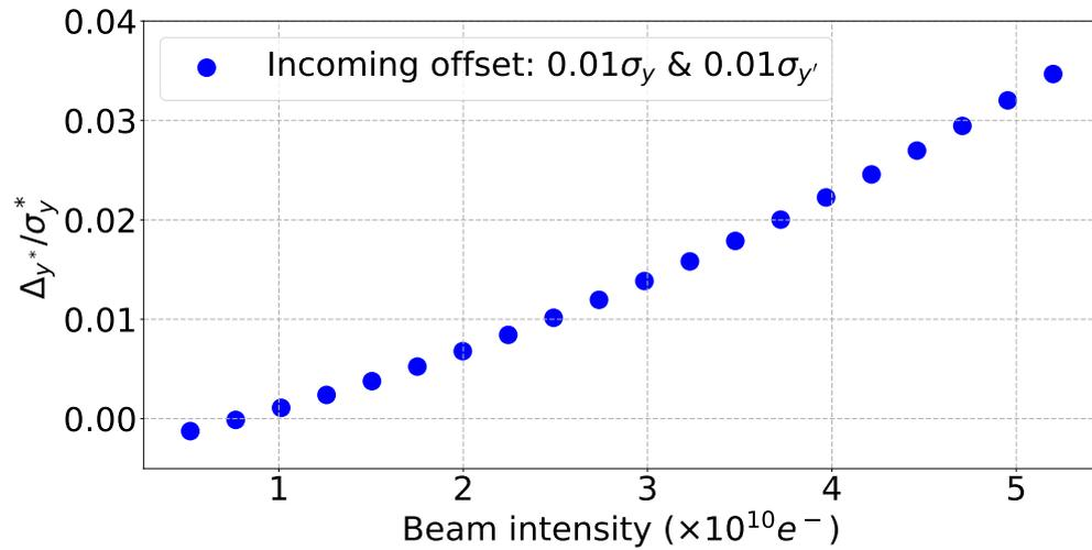
Figure 6.13: Vertical orbit deflection at the IP between the first and last bunch of a train normalised by the IP vertical beam size ( $\Delta y^*/\sigma_y^*$ ) vs. beam intensity for a train with incoming constant horizontal position and angle offsets of respectively  $0.01\sigma_x$  and  $0.01\sigma_{x'}$  and vertical incoming position and angle offsets of respectively  $0.01\sigma_y$  and  $0.01\sigma_{y'}$  in the 380 GeV BDS, calculated with PLACET with resistive walls.
