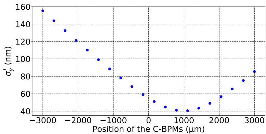
Figure 3.27: Vertical beam size at the IP  $\sigma_y^*$  vs. the position of the bellows, for one machine, calculated with PLACET in the presence of wakefields.
