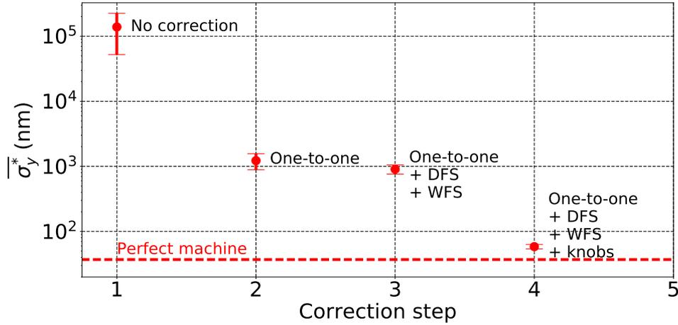
Figure 3.15: Average vertical beam size at the IP ( $\sigma_y^*$ ) vs. correction step: One-to-one, DFS, WFS corrections and IP tuning knobs. The red dashed line show the vertical beam size at the IP for a perfect machine, 37 nm.
