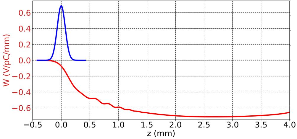
Figure 6.4: Transverse wakepotential in V/pC/mm of the CLIC C-BPM, calculated with GdfidL for a vertical offset of 1 mm, Gaussian bunch length of 70  $\mu\text{m}$  and 1 pC charge (in red). For reference, the distribution of the electrons in one bunch is shown (in blue).
