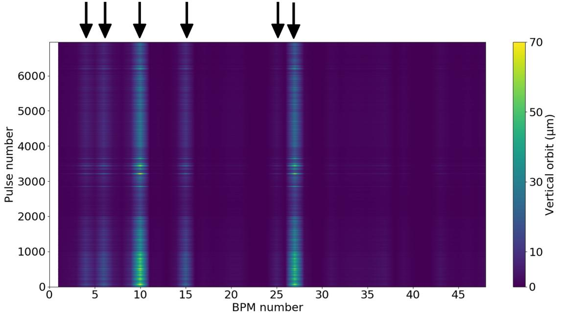
Figure 4.18: Contour plot of the reconstructed matrix  $D_q$  using only the sixth singular value. The arrows show the BPMs having a strong correlation between the measured vertical orbit and the beam intensity.
