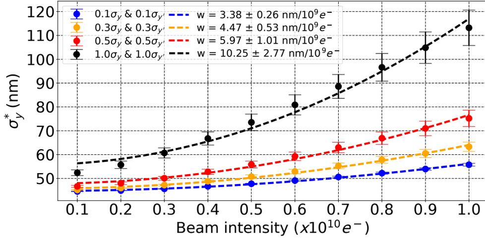
Figure 3.23: Effect of both incoming  $0.1$ ,  $0.3$ ,  $0.5$  and  $1.0$   $\sigma_y$  beam position and  $0.1$ ,  $0.3$ ,  $0.5$  and  $1.0$   $\sigma_{y'}$  beam angle jitters on the vertical beam size at the IP ( $\sigma_y^*$ ) vs. the beam intensity, calculated with PLACET in the presence of wakefields.
