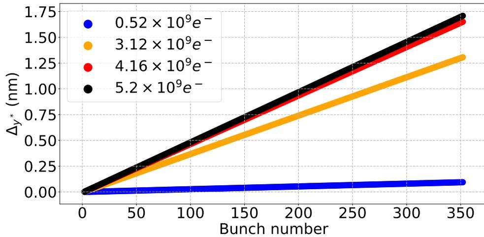
Figure 6.11: Vertical orbit deflection at the IP between the first and last bunch of a train  $\Delta y^*$  vs. bunch number for a train with a constant incoming angle offset of  $0.1\sigma_y$  of the train of bunches in the 380 GeV CLIC BDS, calculated with PLACET with resistive walls.
