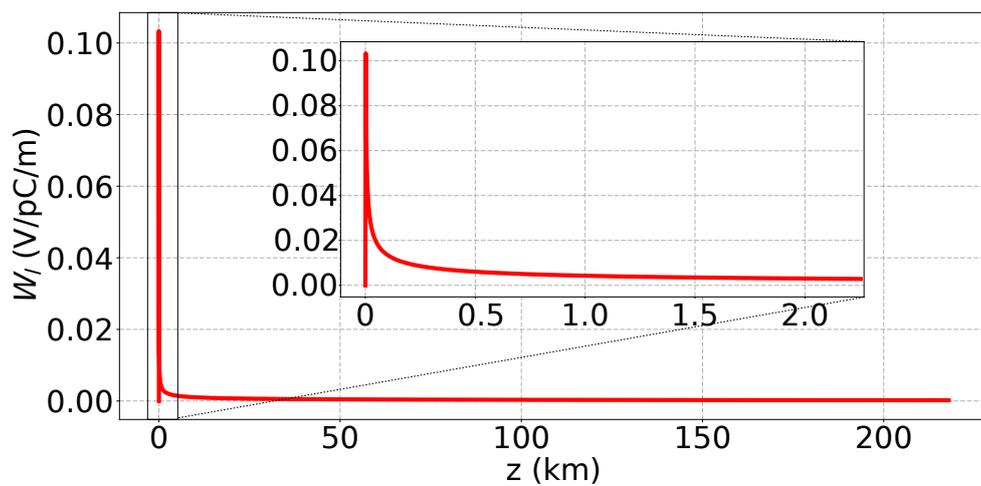
Figure 5.7: The ILC resistive walls wakepotential for a copper beam pipe with a constant radius of 10 mm for the length of a train ( $\sim 218$  km). The zoom shows the wakepotential for the length of the ILC BDS ( $\sim 2254$  m).
