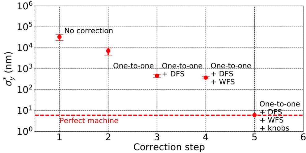
Figure 5.18: Average vertical beam size at the 500 GeV ILC IP ( $\sigma_y^*$ ) vs. correction step: One-to-one, DFS, WFS corrections and IP tuning knobs. The red dashed line show the vertical beam size at the IP for a perfect machine, 5.9 nm.
