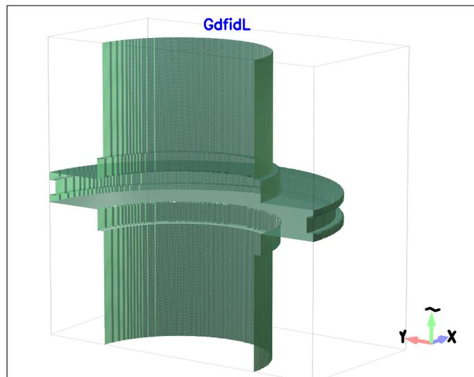
Figure 3.10: The geometry of the ATF2 flange, inputted in GdfidL.
