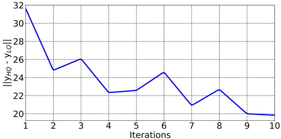
Figure 4.22: Norm of the difference between the vertical orbit at high intensity,  $6.0 \times 10^9$  electrons ( $y_{HQ}$ ) and at low intensity,  $2.0 \times 10^9$  electrons, ( $y_{LQ}$ ) vs. the number of iterations of the WFS correction.
