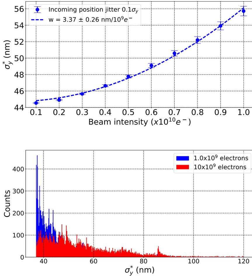
Figure 3.20: (Top) Effect of an incoming  $0.1\sigma_y$  beam position jitter on the vertical beam size at the IP ( $\sigma_y^*$ ) vs. the beam intensity; (Bottom) distributions of the vertical beam size at the IP ( $\sigma_y^*$ ) for low and high beam intensities, calculated with PLACET in the presence of wakefields.
