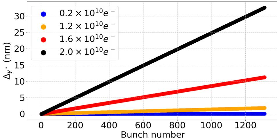
Figure 5.21: Vertical orbit deflection at the IP between the first and last bunch of a train  $\Delta y^*$  vs. bunch number for a train with a constant incoming angle offset of  $0.1\sigma_{y'}$  of the train of bunches in the 500 GeV ILC BDS for 5 beam intensities, calculated with PLACET with resistive wall effects included.
