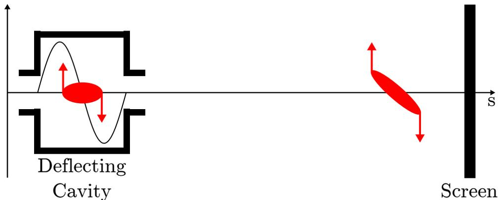
Figure 3.4: A diagram of an RF deflecting cavity being used for bunch length measurement.
