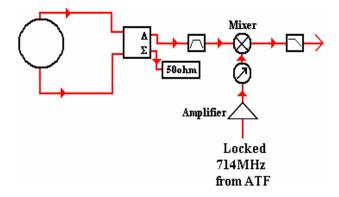
Figure 4: Schematic of BPM signal processor.
