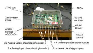
Figure 3: FONT4 digital feedback board.
