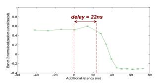
Figure 4: Kick to bunch 2 vs. added delay.
