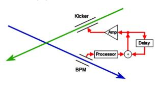
Figure 1: Schematic of IP intra-train feedback system with a crossing angle. The deflection of the outgoing beam is registered in a BPM and a correcting kick applied to the incoming other beam.
