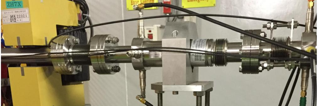
The FONT beam position monitoring system has three 12 cm stripline beam position monitors (BPMs) P1, P2 and P3, each on an x, y mover system. Two further BPMs are used to witness the feedback correction: a stripline BPM (MFB1FF) located ~30 m downstream of P3, and a cavity BPM (IPC) [5] located near the IP.
