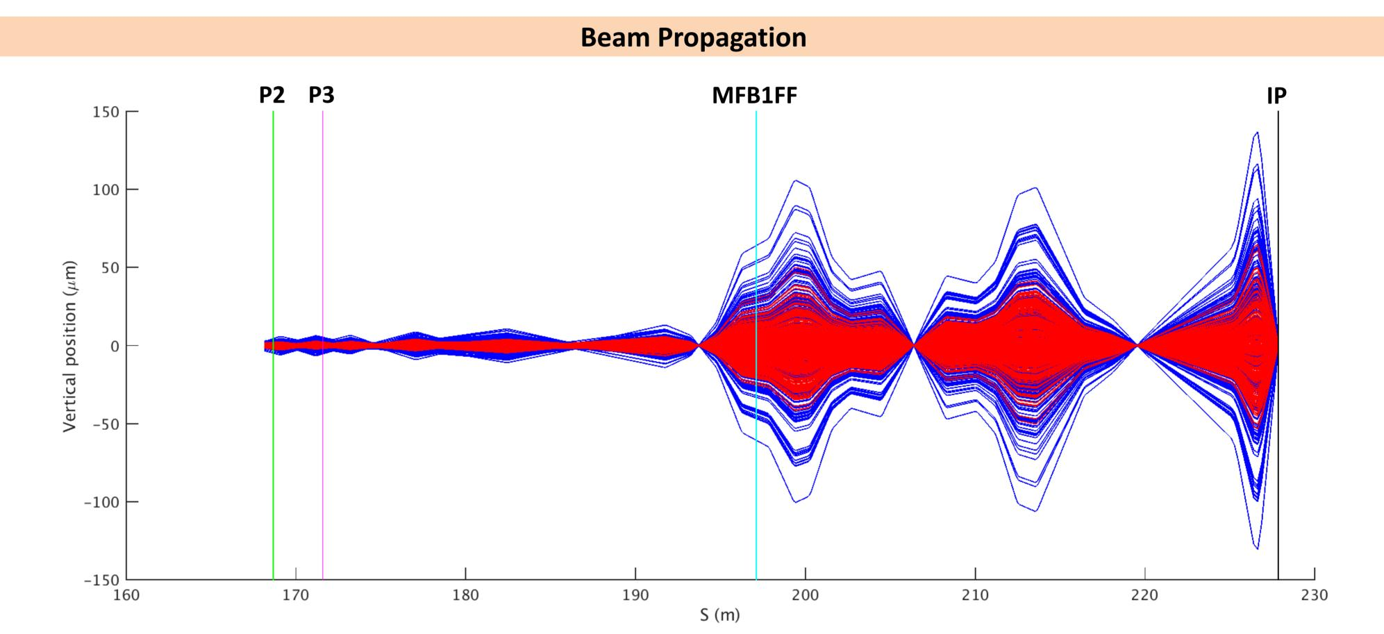
Taking the measured beam position without (blue) and with (red) the application of feedback at P2 and P3 allows the beam to be propagated through the lattice to the ATF IP. As the coupled-loop feedback acts in both vertical betatron phase advances, both the beam position and angle are stabilised downstream of the feedback system.
