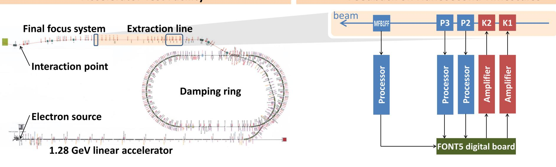
The Accelerator Test Facility (ATF2) [2] at KEK in Japan is a test facility for the ILC and aims to achieve position stability at the notional IP of  $^2$  nm. This goal requires stabilising the beam to under 1  $\mu$ m in the extraction line [3].
