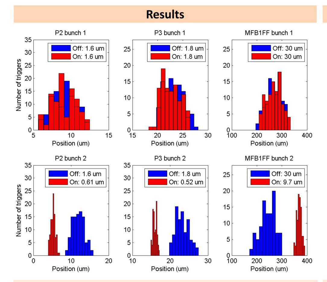
A factor ~3 reduction in the measured position jitter (quoted in the legend) is observed on comparing data without feedback (blue) to data with feedback (red) at P2, P3 and MFB1FF.
