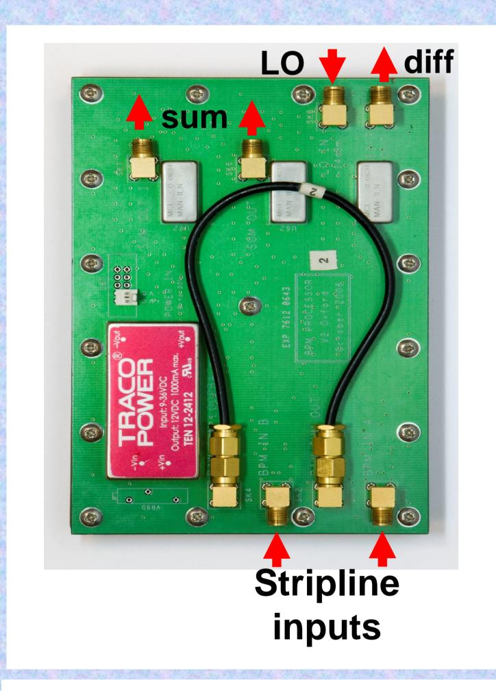
Left: Photo of BPM processor electronics, detailing outputs and major components (right). Stripline BPMs are used for this experiment due to latency restrictions. These tests implement y corrections and so the top and bottom stripline signals are input to the processor. These are subtracted using a hybrid, filtered and down-mixed using a 714MHz local oscillator which is phase-locked to the beam.
