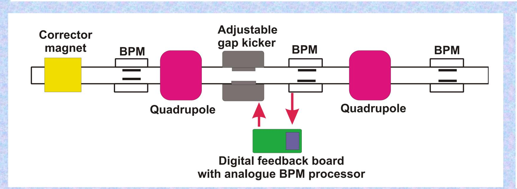
Testing of the FONT feedback system is carried out at the accelerator test facility (ATF) at KEK in Japan. The diagram (left) shows the layout of the system. The BPM output is input to the digital feedback board and the beam position corrected using an adjustable gap kicker.
