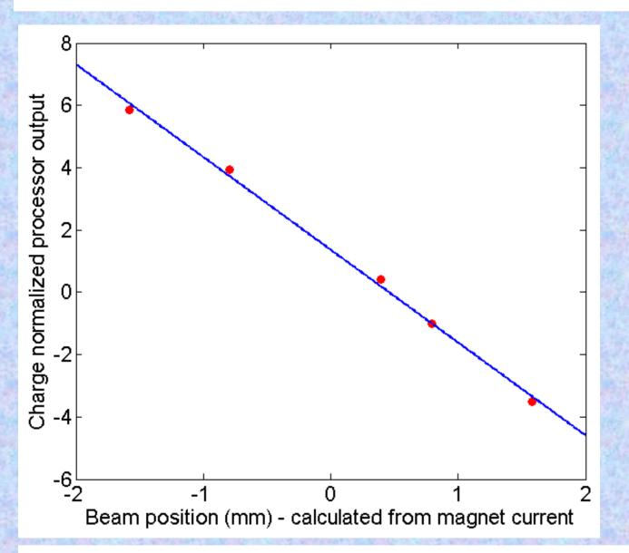
Left: The calibration constant was found to be -3.14mm<sup>-1</sup> which is consistent with the measured gain of the processor.
