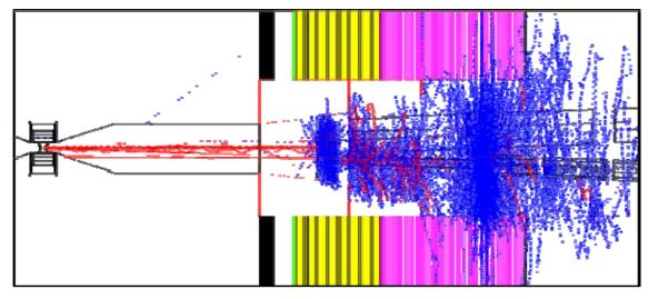
Figure 1: Example simulation of e+e- pairs produced via the beam-beam interaction and tracked through the material model of the IR. Secondary pairs (red lines) and photons (blue lines) are produced in EM showers originating at the mask and at the front face of QFEX1.
