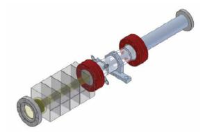
Figure 3: Test module for insertion in ESA beamline showing: low-Z absorber, Beamcal, FB BPM, material model of QFEX1. The total length is 50 inches.
