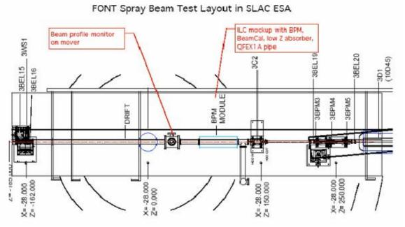
Figure 4: Proposed location for the FONT test module.
