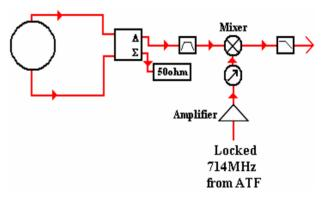
Figure 5: Schematic of BPM signal processor.
