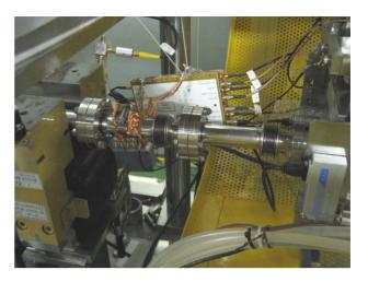
Figure 4: Upstream section of the ATF beamline showing the integrated amplifier and feedback board.
