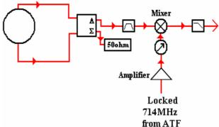
Figure 3: Schematic of BPM signal processor.
