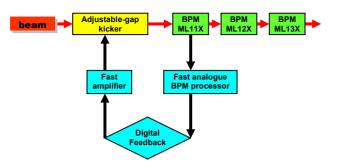
Figure 2: Schematic of FONT4 at the ATF extraction beamline showing the relative locations of the kicker, BPMs and elements of the feedback system.
