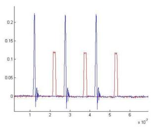
Figure 8: Analogue BPM processor signal (blue) and digital feedback board output (magenta) (V) vs. time (s).
