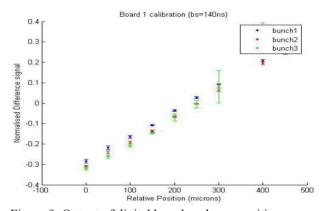
Figure 9: Output of digital board vs. beam position.
