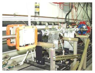
Figure 3: Upstream section of the FONT2 experiment in the NLCTA beamline, showing the dipole magnet for beam steering and the two kickers for beam position correction.
