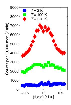
Figure 5.9: Typical fixed-energy Q-scans at E = 5 meV using unpolarised neutrons, showing scans at T = 2,100, and 220 K. Note that the scans are *not* offset from one another.
