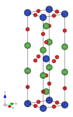
Figure 4.1: The crystal structure of LNSCO [19]. Blue spheres represent  $Cu^{2+}$  ions, red spheres  $O^{2-}$  ions, and green spheres  $La^{3+}$ ,  $Nd^{3+}$  and  $Sr^{4+}$  ions. The space group is  $P4_2/ncm$ .
