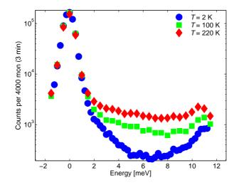
Figure 5.8: Fixed-Q energy scans at  $\mathbf{Q} = (1, 0.5, 0.5)$  using unpolarised neutrons, showing scans at T = 2, 100, and 220 K on a logarithmic scale.
