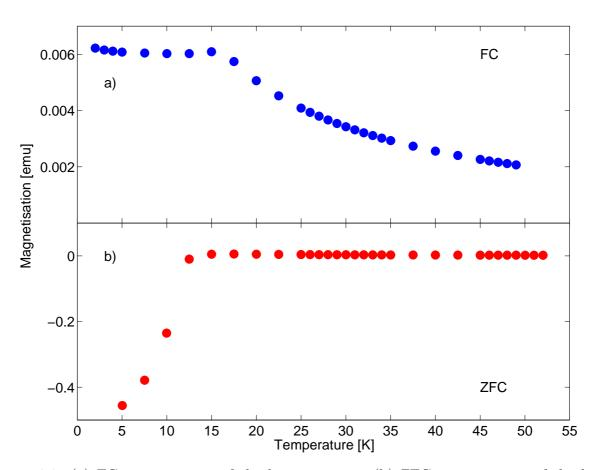
Figure 4.6: (a) FC measurement of the long moment. (b) ZFC measurement of the long moment. The applied magnetic field was 500 Oe in the *ab*-plane.
