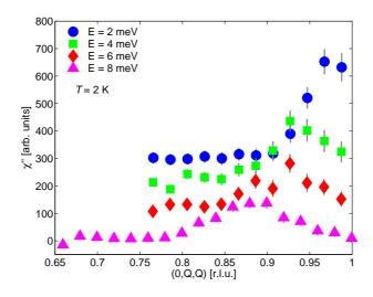
Figure 6.8: Constant energy Q-scans of the magnetic scattering (NSF-SF). T = 2 K. Successive scans are displaced by 100 for clarity.
