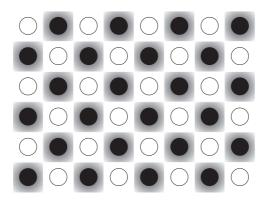
Figure 1.5: Schematic of a charge checkerboard for a half-doped  $La_{2-x}A_xMO_4$  material, with circles representing ions on a square lattice and the shading representing localised charge.
