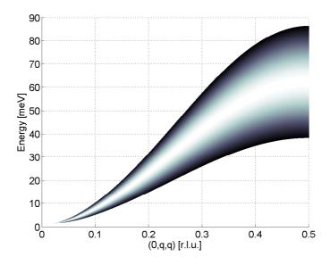
Figure 6.16: Broadening of the dispersion due to a Gaussian distribution of nearest-neighbour exchange parameters.
