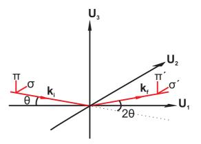
Figure 2.8: The coordinate system used for defining the scattering plane and the components of magnetic moments in the resonant scattering cross sections.  $\pi$  and  $\sigma$  are the components of the polarization parallel and perpendicular to the scattering plane respectively.
