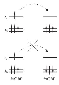
Figure 6.1: The double exchange mechanism. In the upper half the ferromagnetic case is shown, where electron hopping is possible. In the lower half of the figure the antiferromagnetic case is shown, where hopping is not possible
