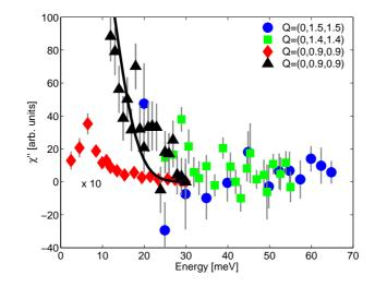
Figure 6.14: Fixed wavevector energy scans, comparing a scan at (0, 0.9, 0.9) where there is a clear spin-wave peak, with scans at (0, 1.4, 1.4) and (0, 1.5, 1.5), where there is no apparent signal. The scan at (0, 0.9, 0.9) is shown twice, black triangles and the black line show it to scale with a fit, whereas red diamonds show it reduced by a factor of 10.
