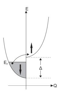
Figure 1.7: The split spin bands in a Fermi gas (metal), showing a single particle spin-flip excitation from one band to another. Arrows denote the spin state in each band.
