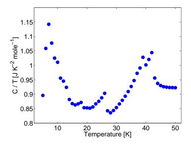
Figure 7.8: Measurement of the heat capacity of the crystal of  $DyMn_2O_5$  used in the x-ray measurements. The temperatures at which there are anomalies agree with those measured previously [2, 4]. Note that the lattice heat capacity has not been subtracted from these data.
