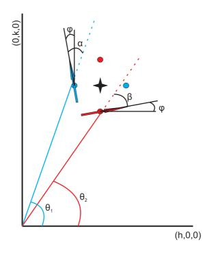
Figure 4.24: Definitions of angles used in analysis of the polarised neutron diffraction data.
