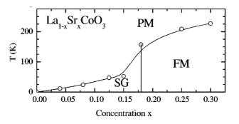
Figure 6.4: (After Kriener *et al* [5])The magnetic phase diagram of  $La_{1-x}Sr_xCoO_3$ , showing the spin glass (SG), paramagnetic (PM), and ferromagnetic (FM) phases.
