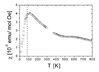
Figure 5.1: After English *et al* [1], the magnetic susceptibility of  $LaCoO_3$  as a function of temperature. Van-Vleck and impurity contributions to the susceptibility have been subtracted from these data.
