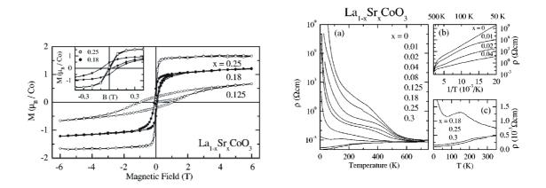
Figure 6.3: Left-hand panel (after Kriener *et al* [5]), magnetic susceptibility of  $\text{La}_{1-x}\text{Sr}_x\text{CoO}_3$  as a function of applied magnetic field and doping x. Right-hand panel (after Kriener *et al* [5]), resistivity of  $\text{La}_{1-x}\text{Sr}_x\text{CoO}_3$  as a function of temperature and doping x.
