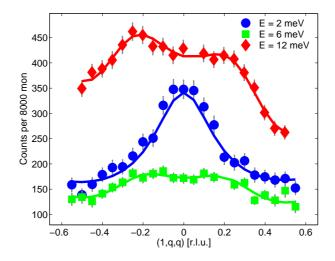
Figure 5.10: Fits to equation 5.2, plus a sloping background since the data were not fully polarisation-analysed, of fixed energy Q-scans with  $\mathbf{P} \parallel \mathbf{Q}$  spin-flip, taken with the Oxford sample on IN20 at T = 220 K. Note that the data at E = 12 meV was taken with  $k_f = 4.1 \text{ Å}^{-1}$ , whereas the other two scans were with  $k_f = 2.662 \text{ Å}^{-1}$ .
