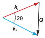
Figure 2.2: The scattering triangle, relating the incident and final wavevectors to the scattering wavevector
