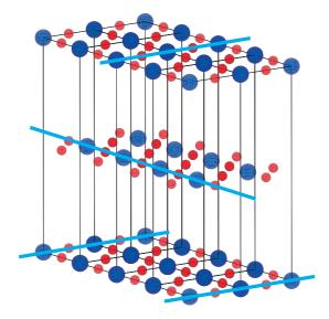
Figure 4.2: A schematic of the charge order in a tetragonal unit cell proposed by the stripe model
