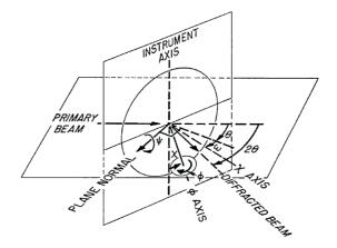
Figure 2.4: After Busing and Levy. All of the angles shown here for the four-circle diffractometer are in their first quadrant.
