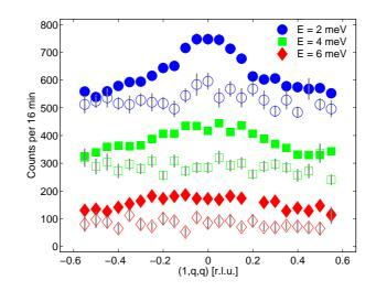
Figure 5.2: Fixed-energy Q-scans for  $\mathbf{P} \parallel \mathbf{Q}$ , spin-flip (filled symbols) and non-spin-flip (open symbols), showing the magnetic scattering at T = 220 K with energies in the range  $2 \leq E \leq 6 \text{ meV}$ . Scans at successive energies are offset by 200. The Oxford-grown sample was used for these measurements.
