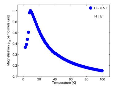
Figure 7.7: The magnetisation of  $DyMn_2O_5$  as a function of temperature in an applied field of 0.5 T parallel to the *b*-direction.
