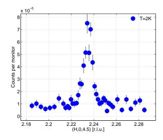
Figure 4.18: Scan of charge-order induced structural distortion peak in LBCO, at T=2 K in zero applied field.
