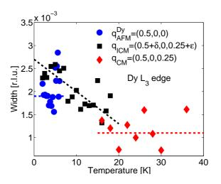
Figure 7.12: The widths (FWHM) of the peaks corresponding to the Dy AFM, ICM and CM order measured in scans parallel to (0, 0, L). The widths were determined by moment analysis. The dashed lines are guides to the eye. Similar analysis of scans parallel to (H, 0, 0) and (0, K, 0) (not shown) shows no change in the width in these directions.
