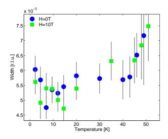
Figure 4.22: The temperature dependence of the width of the charge order induced structural peak at  $\mathbf{Q} = (2.24, 0, 4.5)$  in LBCO with zero applied magnetic field, and an applied field of 10 T.
