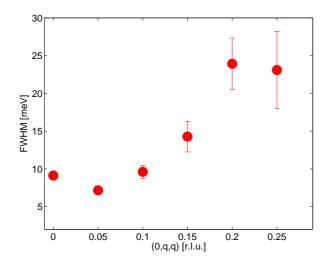
Figure 6.11: Full width at half maximum (FWHM) in energy of the magnetic excitations as a function of wavevector.
