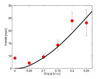
Figure 6.17: The expected width of the spin excitations if the exchange parameter has random disorder (black line), plotted over the real energy width of the spin excitations (filled red circles).
