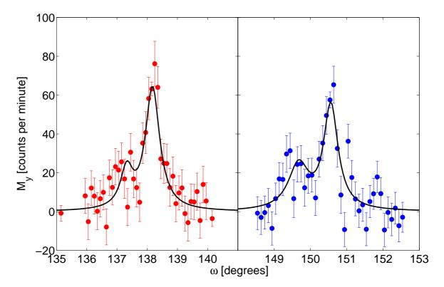
Figure 4.9: Polarisation analysed  $\omega$  -scans with T = 10K at  $\mathbf{Q} = (0.5, 0.62, 0)$  and  $\mathbf{Q} = (0.62, 0.5, 0)$ , denoted by red and blue circles respectively. The y-axis corresponds to the magnetic signal arising from ordered moments that are in-plane and perpendicular to the scattering wavevector. The black line represents a fit to the data, described in the text.
