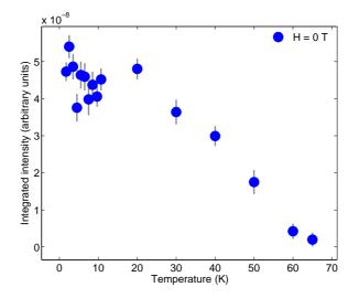
Figure 4.19: The temperature dependence of the integrated intensity of the charge order induced structural peak at  $\mathbf{Q} = (2.24, 0, 4.5)$  in LNSCO.
