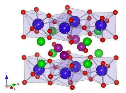
Figure 7.2: The unit cell of  $DyMn_2O_5$ , with Dy ions shown as blue spheres,  $Mn^{4+}$  ions shown as purple spheres,  $Mn^{3+}$  ions shown as green spheres, and  $O^{2-}$  ions shown as red spheres. The polyhedra show the  $DyO_8$  neighbours.
