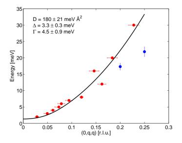
Figure 6.12: Damped harmonic oscillator fit to the low energy spin-waves, assuming a quadratic dispersion. The raw data have been fitted in this case.
