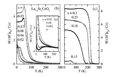
Figure 6.2: (After Kriener *et al* [5]) Magnetic susceptibility of  $La_{1-x}Sr_xCoO_3$  as a function of temperature and doping x.
