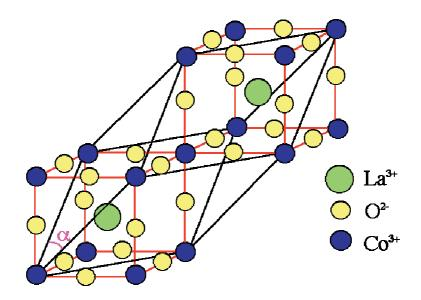
Figure B.1: The (non-primitive) unit cell of LaCoO<sub>3</sub>, which is rhombohedral. Since the angle  $\alpha$  is only slightly greater than 60° in this material the distortion away from cubic (for which  $\alpha=60^{\circ}$ ) is also small.
