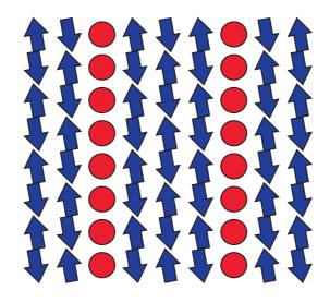
Figure 4.3: A schematic of a single  $CuO_2$  plane showing the spin ordering proposed in the stripe model.
