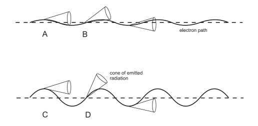
Figure 2.3: A schematic of an undulator (upper figure) and a wiggler (lower figure) insertion device. The cones shown at various points along the electron path show the direction of the emitted radiation.
