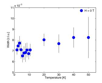
Figure 4.21: The temperature dependence of the width of the charge order peak in LNSCO in zero applied magnetic field
