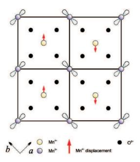
Figure 1.6: (After Wilkins *et al* [17], schematic of orbital order in  $La_{0.5}Sr_{1.5}MnO_4$ .
