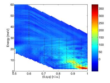
Figure 6.6: Colour map showing the magnetic scattering (NSF-SF), all scans combined and symmetrised. T = 2 K.
