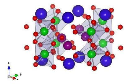
Figure 7.4: The  $DyMn_2O_5$  unit cell showing  $Mn^{3+}O_6$  octahedra
