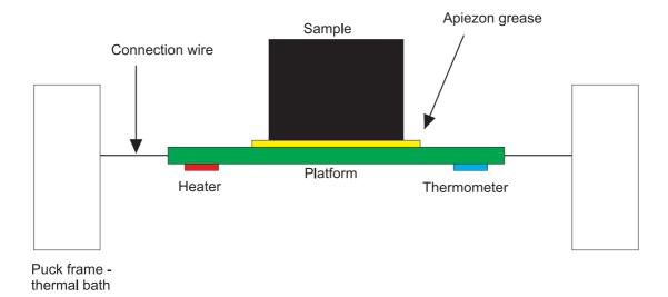
Figure 2.10: Side view of the sample mount for heat capacity measurements using the PPMS
