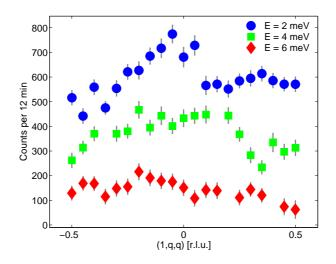
Figure 5.5: Fixed-energy Q-scans after polarisation analysis, showing the magnetic scattering at T = 220 K for  $2 \le E \le 6$  meV. Successive scans have been offset by 200 for clarity. The Cologne-grown sample was used for these measurements.
