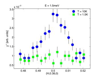
Figure 4.12: Fixed-energy wavevector scan over the (0.5, 0.38, 0) position with E = 1.5 meV, showing the scattering at T = 1.5 K and T = 10 K.
