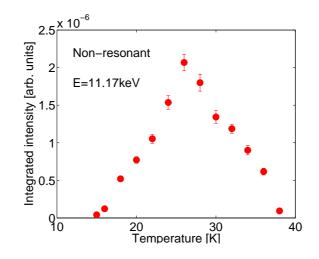
Figure 7.13: Temperature variation of the intensity of the signal at  $\mathbf{q} = (0, 0, 0.5)$  measured with a non-resonant x-ray energy. The intensities were calculated from fits to a Gaussian for scans parallel to (H, 0, 0). This scattering is structural in origin.
