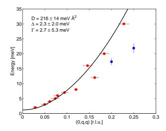
Figure 6.13: Damped harmonic oscillator fit to the low energy spin-waves, assuming a quadratic dispersion. The processed data have been fitted in this case.
