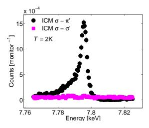
Figure 7.11: Scans of the incident x-ray energy for the ICM signal at  $(0.5 + \delta, 0, 0.25 + \epsilon)$ . The strong peaks in the  $\sigma - \pi'$  channel, together with a lack of signal in the  $\sigma - \sigma'$  channel, shows that the scattering is purely magnetic at this wavevector.
