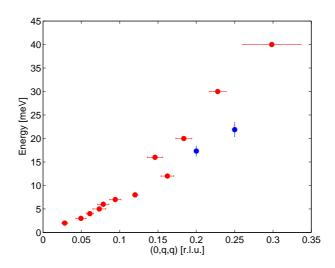
Figure 6.10: Fits to Q- and E-scans to determine a dispersion relationship. Red filled circles with horizontal errorbars are determined from Q-scans, blue filled circles with vertical errorbars are from E-scans.
