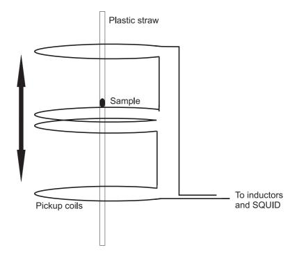
Figure 2.9: The pickup coils of the SQUID magnetometer.
