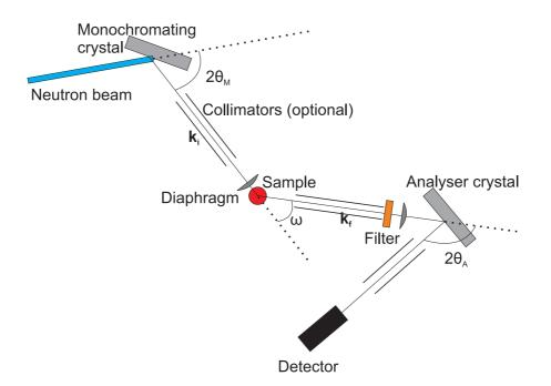
Figure 2.1: A schematic of a conventional triple-axis spectrometer.
