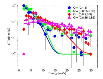
Figure 6.9: Fits to fixed-wavevector energy scans, using a single Gaussian. T = 2 K. Note that all of the data points and fits have been offset by +1 so that a logarithmic scale can be used.
