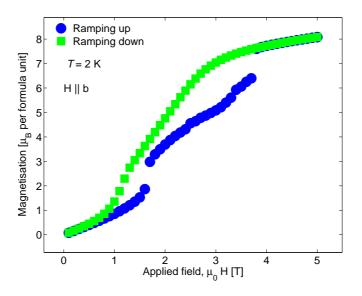
Figure 7.6: Measurement of the magnetisation at T = 2 K, with the applied magnetic field, which was parallel to the *b*-direction, being ramped up (blue circles) and ramped down (green squares). On ramping the field up there are jumps in the magnetisation at about 1.7 T and 3.7 T, however these transitions do not occur when the field is ramped down.
