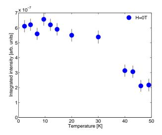
Figure 4.20: The temperature dependence of the integrated intensity of the charge order induced structural peak at  $\mathbf{Q} = (2.24, 0, 4.5)$  in LBCO.
