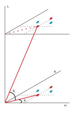
Figure 4.15: The scattering planes used for the second measurement on the IN14 spectrometer.
