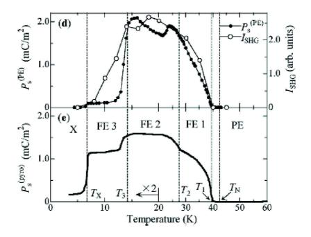
Figure 7.1: FE polarisation measured by Higashiyama *et al.* [4]. The upper figure shows remnant polarisation after the applied electric field has been cycled, analogous to a magnetic hysteresis loop. The lower figure shows the polarisation inferred from measurement of the pyroelectric current.
