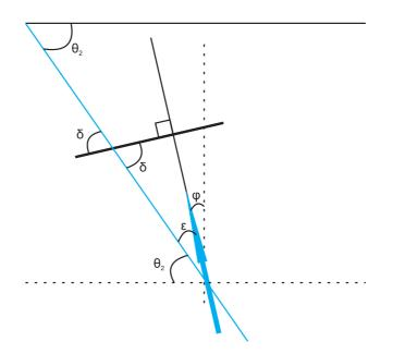
Figure 4.26: Definitions of the second set of angles used in analysis of the polarised neutron inelastic scattering data.
