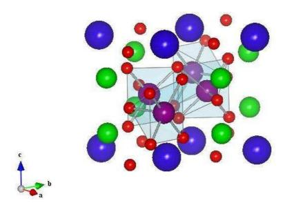
Figure 7.5: The  $DyMn_2O_5$  unit cell showing  $Mn^{4+}O_5$  bi-pyramids
