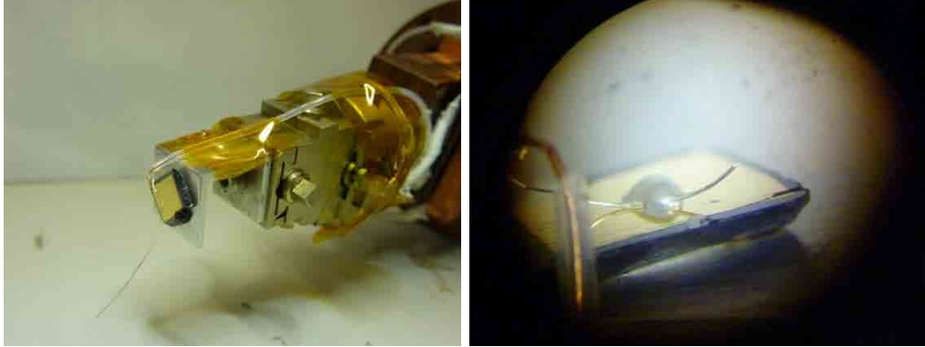
Figure 6.8: Sample setup for spherical neutron polarimetry measurements on MuPAD/TASP. The left panel shows the sample mounted on a goniometer and attached to the sample stick. The right panel is a view of the electrode attached to the surface of the sample by Ag epoxy.
